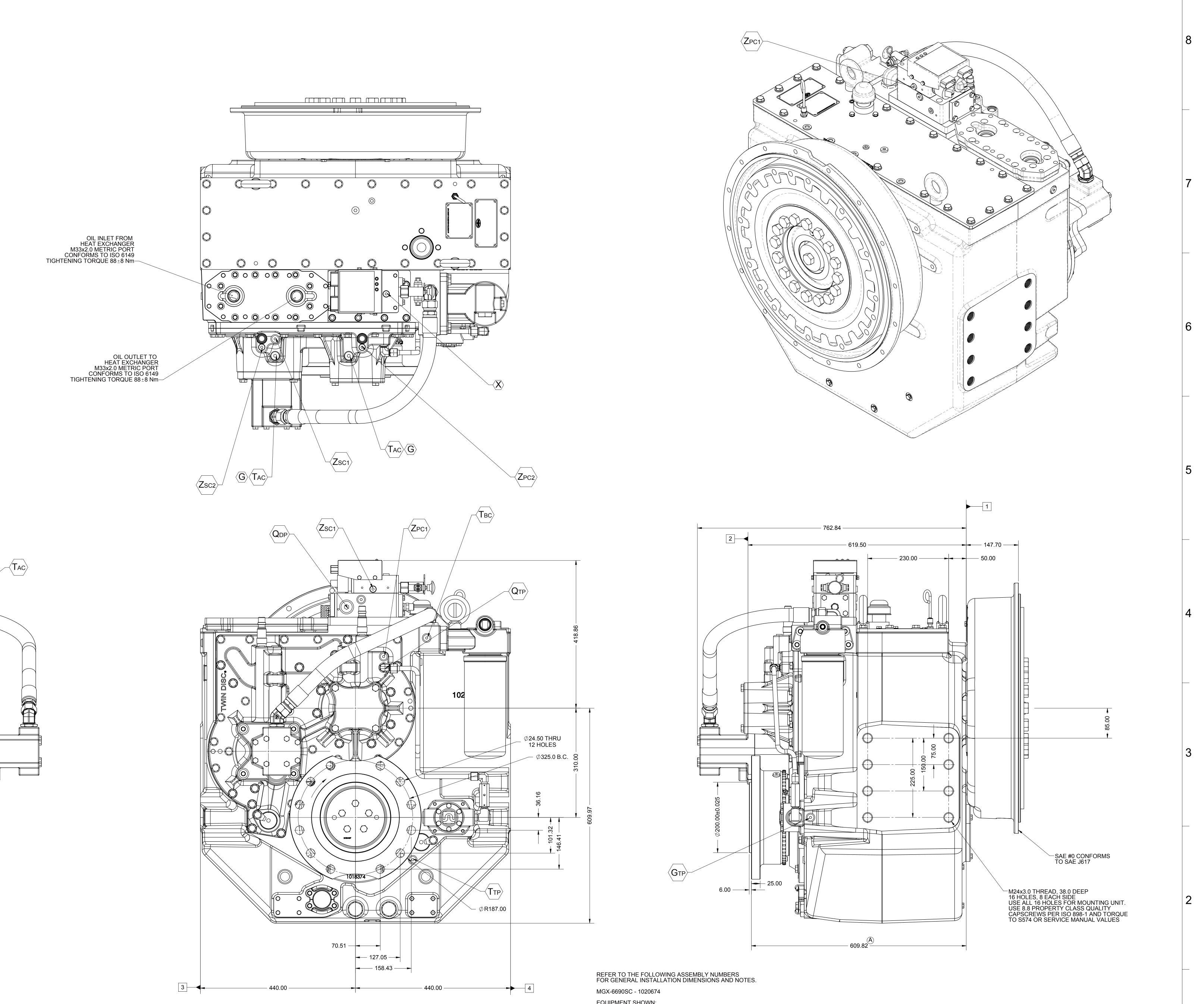
EQUIPMENT SHOWN: -INPUT GROUP 1025088B -GP VALVE WITH EC050 MODULE -DITCHPLATE FOR CUSTOMER SUPPLIED HEAT EXCHANGER -TRAILING PUMP
