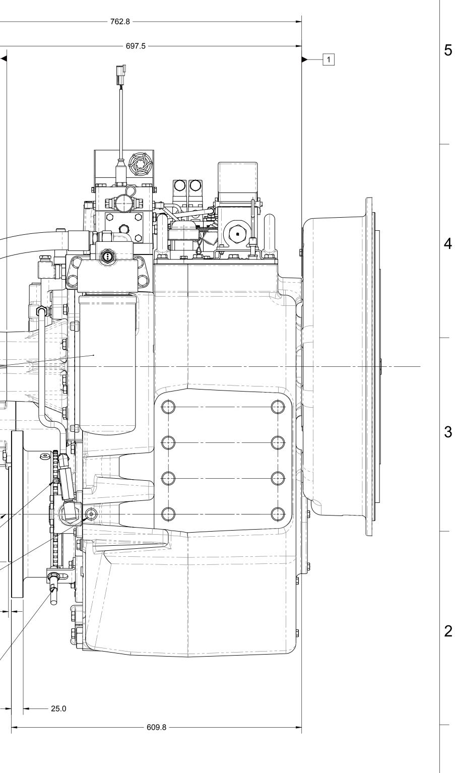
EQUIPMENT SHOWN: - SAE #0 APPLICABLE MODELS: MGX-6690SC PER 1020674 ASSEMBLY - SAE 460 CENTA CF-R-520-HR COUPLING - GP VALVE WITH EC300 HARNESS MGX-6848SC PER 1020675 ASSEMBLY - RAW WATER HEATE EXCHANGER - TRAILING PUMP NDWF-04792 05/14/2014 - SAE J744 127-2/4, 32-4 OR 38-4 LIVE PTO - 1024843X BLUE VISION - NG BASIC MONITORING GROUP REV CHANGE NO. DATE WEIGHT:1026.15kg THIRD ANGLE PROJECTION MATERIA (TWIN((DISC) 01/20/2014 SCALE
