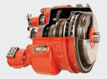
**TORQUE CONVERTERS** By transmitting torque through fluid mass in motion, Twin Disc converters eliminate mechanical connections and reduce or eliminate the need for shifting, clutching and declutching.
