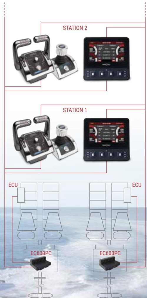
System example shows a non-redundant setup for a twin engine installation with two stations.
