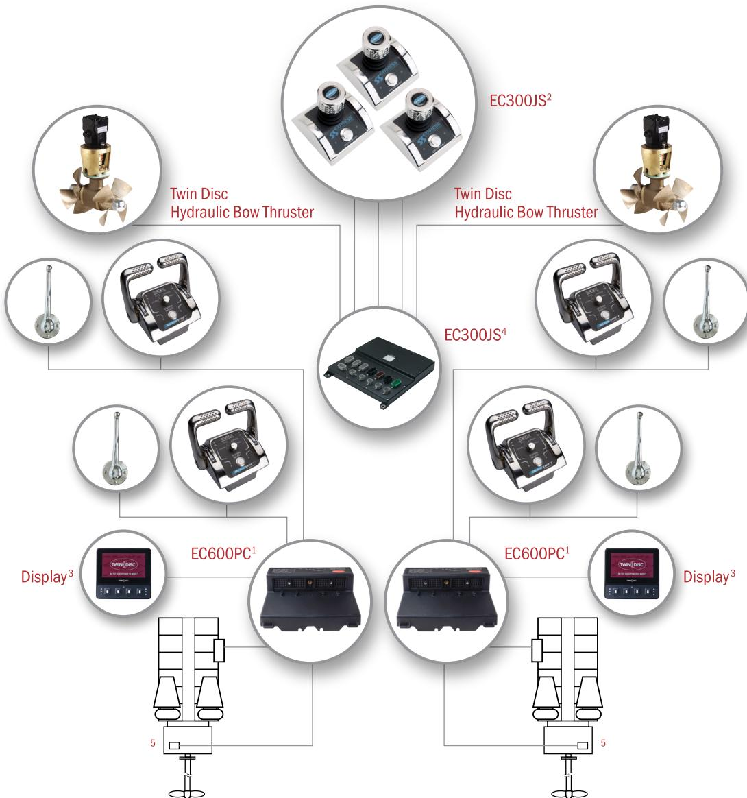
1 EC600PC: Standard control system for up to seven digital stations and up to eight engine/transmission shaft lines per vessel.
