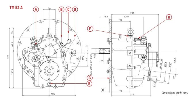
A Neutral indicator **B** Oil from cooler **C** Dipstick **D** Oil to cooler **E** Drain plug **F** Vent **G** Mounting flange **H** Actuating lever
